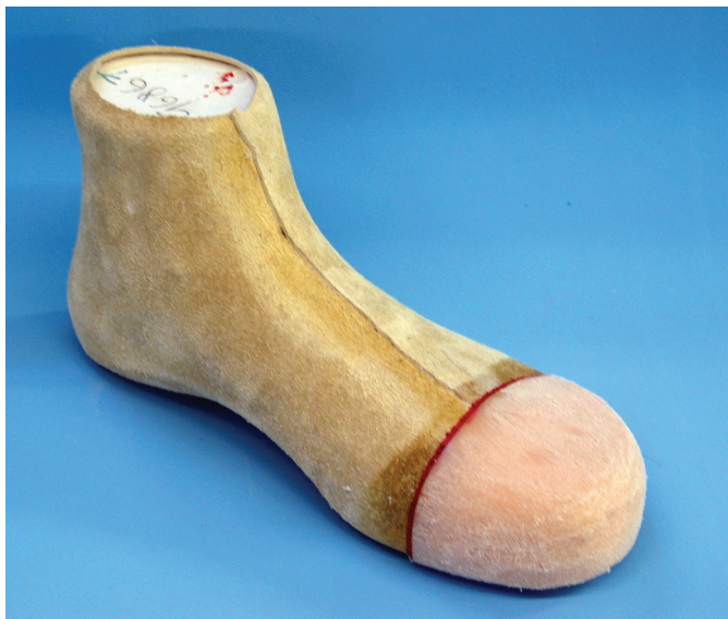
Thermoplastic safety toe box over leather lining on modified shoe last.
